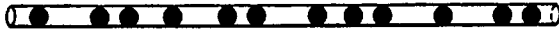
Fig. 2. Representation of a phason imperfection as a flex comprising point excitations (whose properties are close to those of grain boundary impurities).
